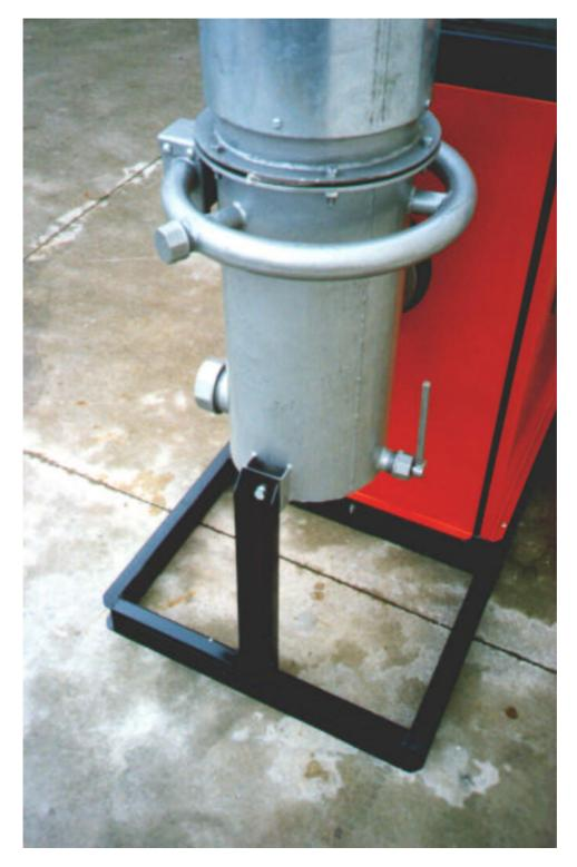
This was the original size of the Pioneer Class hearth and fuel hopper, but the narrow hopper caused fuel flow problems. We fitted a larger hopper, hence the taper on the drawing above the nozzles. It is easier to just have the larger parallel cylinders.
