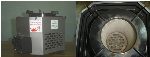
Figure 5: The Oorja stove (a) notice the power pack towards the left bottom section of the left plate (b) the ceramic combustion chamber with grate at the bottom and secondary air holes towards the top
