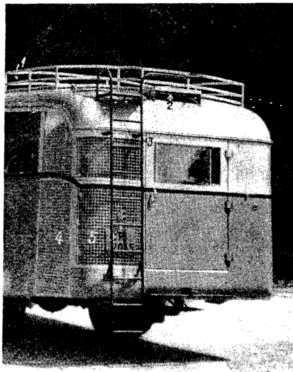
Figure 131. Mail Bus (Switzerland) with the Wood Gas Generator Entirely Enclosed.
