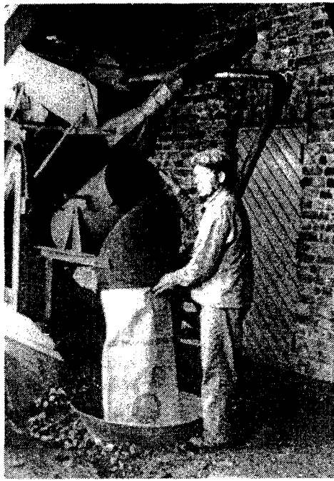
Figure 59. Packing Generator Gas Charcoal
