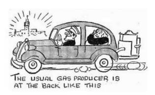
Usually, trucks had the units mounted on the side, behind the doors. A mounting forward of the radiator was available and sometimes on either side of the cabin, forward of the doors. The use of GPU's in the trucking fleet appeared to be quite widespread and was an enforced government policy within its own fleet (eg Forest Commission, Tramways and Victorian Railways etc).
