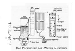
The weight of the typical GPU was between 400-500 lbs (empty) for a passenger vehicle unit. Add another 50-100 lbs for the charcoal.
