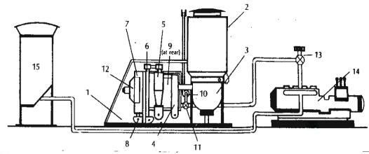
Fig. 1 - Layout of typical Fluidyne gasifier plant showing (1) Supporting frame, (2) Wood fuel container, (3) Hearth, (4) expansion chamber (coarse particles), (5) Multi Cyclone, (6) saturating cooler, (7) condensing cooler, (8) condensate tank, (9) volume filter, (10) start-up fan, (11) change-over valve, (12) gas cooler fan, 13 engine gas/air mixer controller, (14) engine/generator set, (15) wood drier using waste heat.
