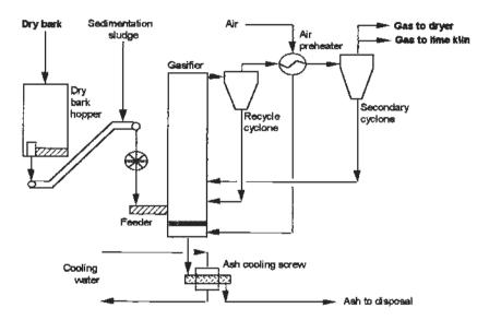
Figure 1 - Lurgi CFB Gasification System at Pöls Pulp Mill [Herbert, 1989]
