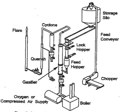
Figure 2 - Layout of Renugas process development unit (PDU)
