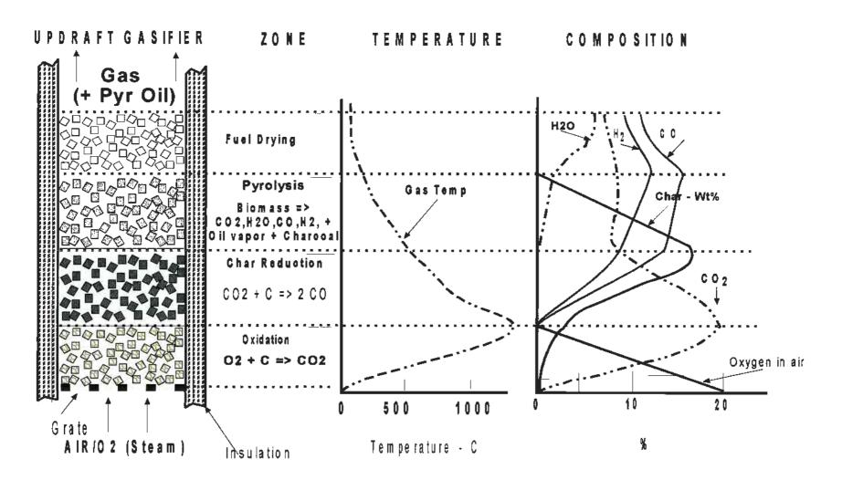
Fig. 2- Schematic diagram of an updraft gasifier showing the gasifier zones, the reactions, the temperatures and the gas composition (zone height not necessarily to scale). Air or oxygen passes up through a grate and burns charcoal, generating very high temperature CO<sub>2</sub> in the oxidation zone; the CO<sub>2</sub> is then reduced to CO (endothermic, gas cools) in the reduction zone; the hot gas then pyrolyses and dries the incoming fuels.
