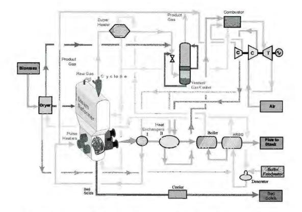
Figure 3: Schematic of the Integrated Steam Reformer/Gas Turbine System for **Power Generation**
