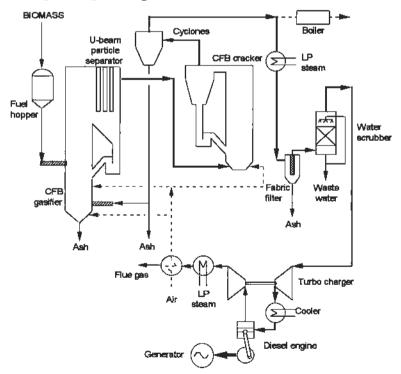
Figure 1 - Flowsheet of Studsvik Atmospheric Gasification Pilot Plant [Annon, 1992]
