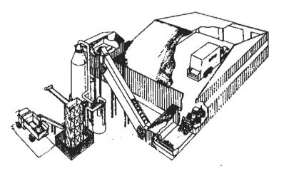
Figure 1 Diagrammatic sketch of the Purox oxygen slagging gasification system
