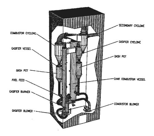
Figure 2 – Layout of Burlington Electric Double Fluid Bed pyrolytic Gasification System
