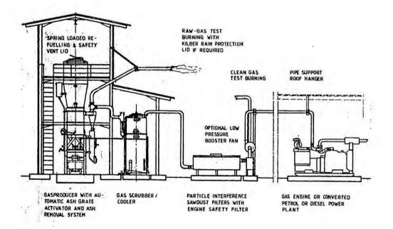
Fig. 2 - General arrangement of SJG gasifier for engine applications
