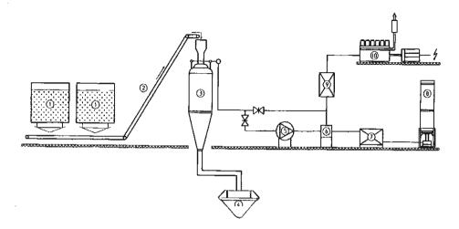
Fig. 1. Schematic of HTV gasification plant showing (1) Fuel container, (2) Fuel feed, (3) Juch-Gasifier, (4) char-ash container, (5) flare fan, (6) condensate reservoie, (7) gas cooler, (8) Gas flare, (9) gas cleaning, (10) motor generator.
