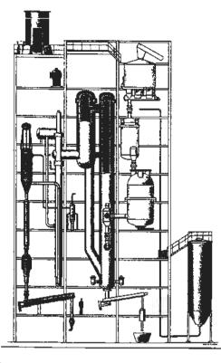
Figure 2 - Arrangement of Varnamo IGCC plant (from report)
