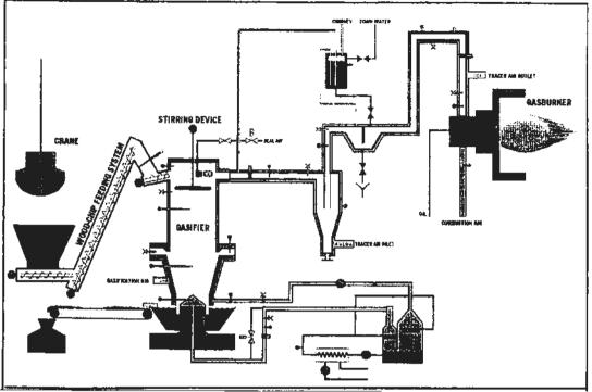
Figure 1 - Flow diagram of the Vølund Harboore Gasifier Plant
