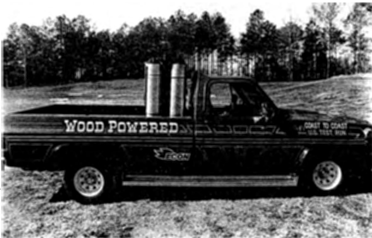
Figure 1. The ECON wood gas producer resulting from a privately funded development program started in 1978. The compact, modular gas producer system weighing 350 pounds is conveniently mounted in the pick-up bed. Commercial production is planned for 1981. Courtesy ECON (The Energy Conservation Company), P.O. Box 828, Alexander City, Alabama 35010.
