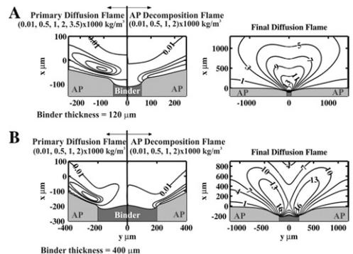
Fig. 4. Predicted gas phase reaction rate ( $\text{kg}/\text{m}^3$ ) contours at pressures of 0.092 MPa for (A) binder thickness of 120  $\mu\text{m}$ , (B) binder thickness of 400  $\mu\text{m}$ .
