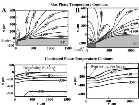
Fig. 5. Predicted gas phase and condensed phase temperature contours for a binder thickness of 120  $\mu\text{m}$  (A) and 400  $\mu\text{m}$  (B) at 0.092 MPa.
