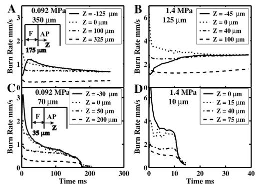
Fig. 6. Predicted burn rates at different cross-sections on the surface parallel to AP–binder interface (distances measured from AP–binder interface) for various cases as indicated.
