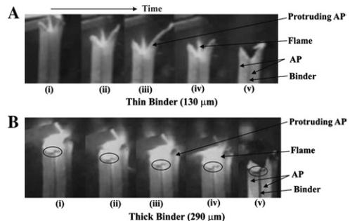
Fig. 3. Experimentally obtained pictures of sandwich burning at 0.092 MPa for binder thicknesses of 130  $\mu\text{m}$  (A) and 290  $\mu\text{m}$  (B). The region inside the ring shows the dark regions adjacent to the binder at the base of the flame.
