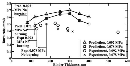
Fig. 2. Predicted variation of sandwich burn rate with binder thickness at two different near atmospheric pressures along with experimentally observed variation of the same.
