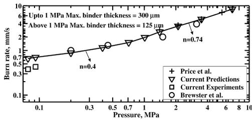
Fig. 7. Predicted variation of burn rate with pressure at large binder thickness (indicated) for sandwich propellant along with experimental results.
