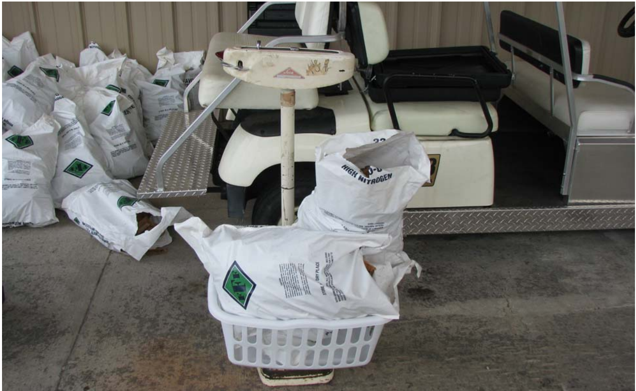
Figure 6. Weighing wood in plastic bags prior to loading into gasifier
