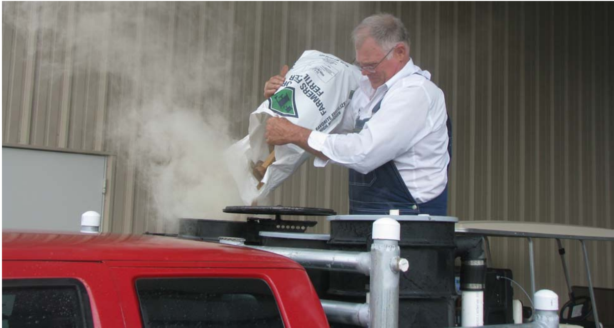
Figure 7. Loading wood into the gasifier
