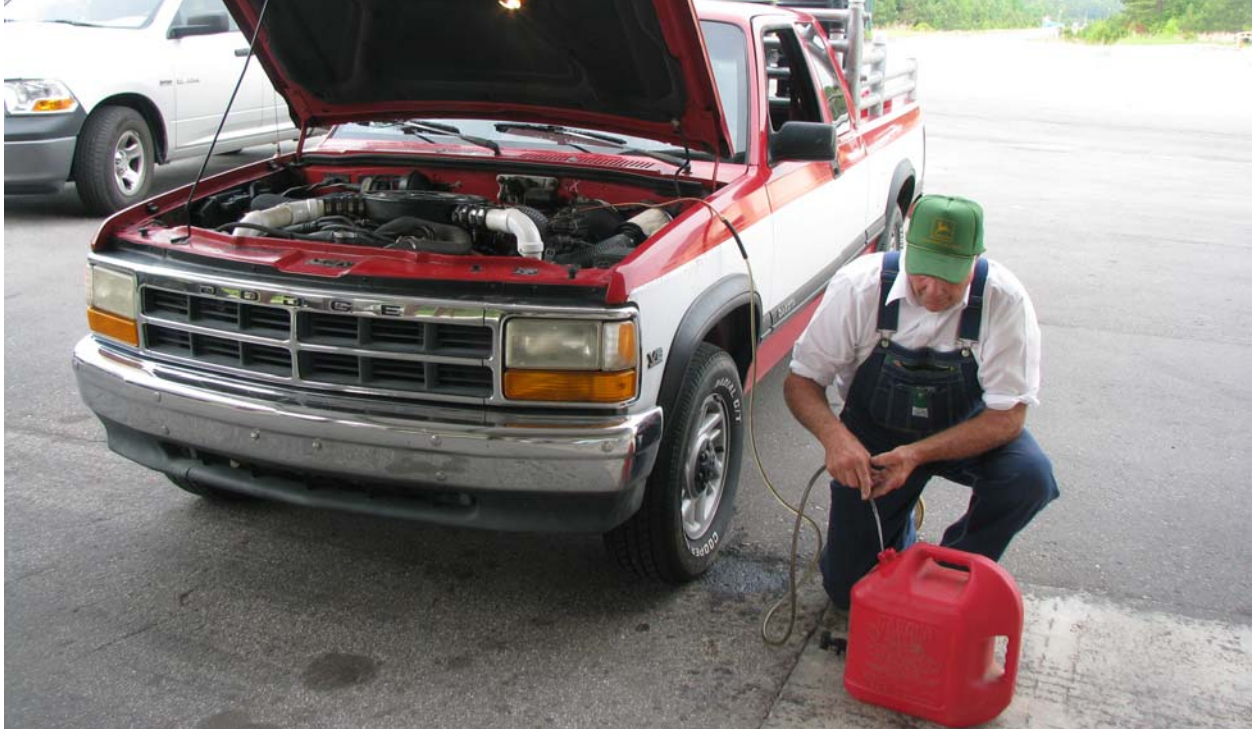
Figure 5. Draining the gas tank prior to the gas test.
