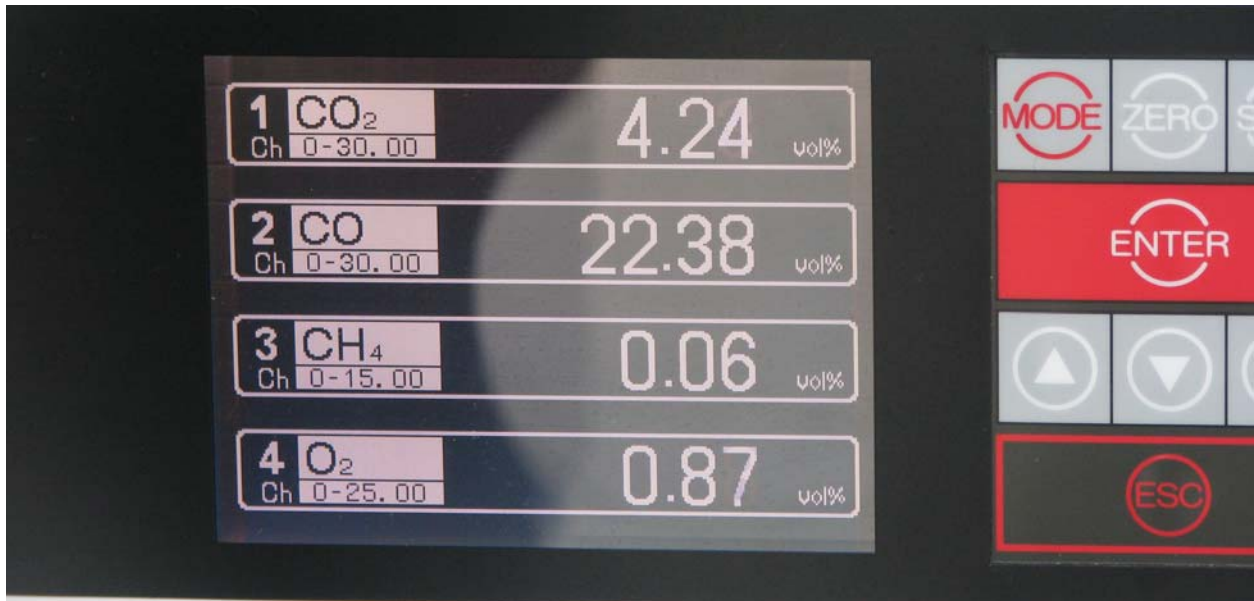
Figure 11. Readings on gas analyzer
