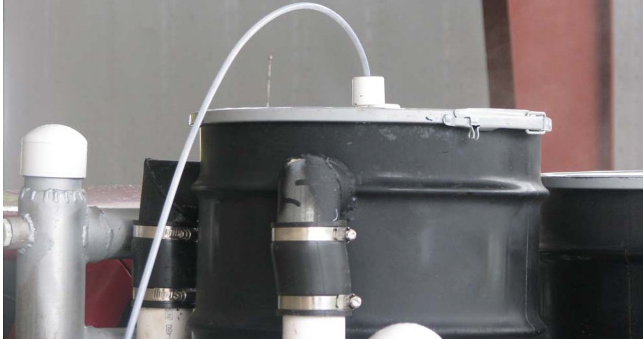
Figure 9. Tube taking syngas sample from gasifier
