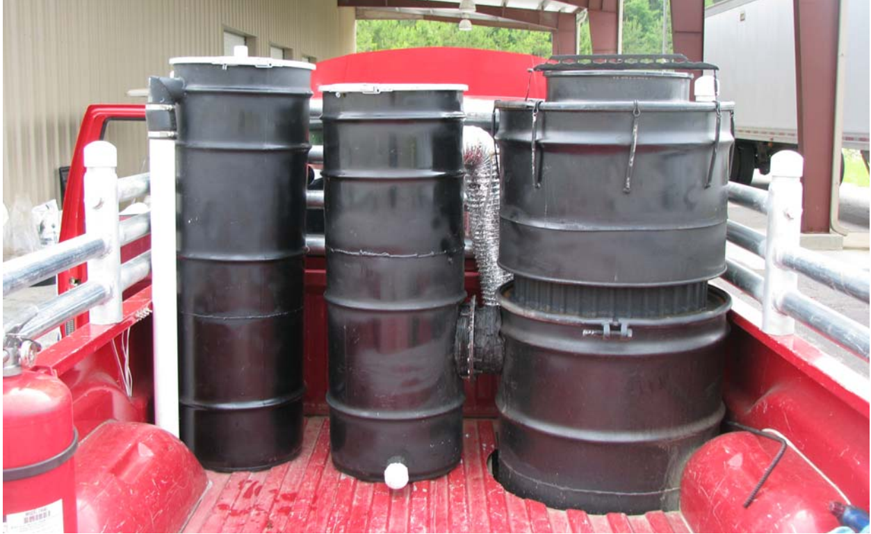
Figure 1. Pick-up mounted down draft gasifier.
