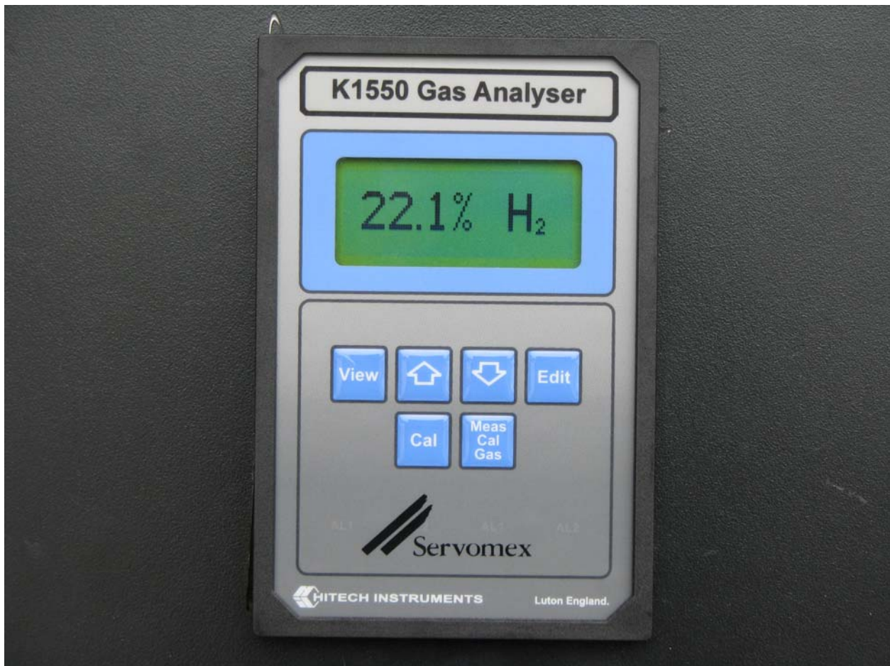
Figure 12. Hydrogen reading on gas analyzer.
