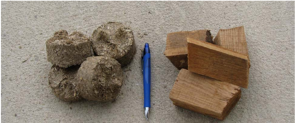
Figure 2. Switchgrass cubes and wood samples.
