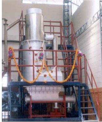
A 75 kW gasification system at an National Institute of Engineering, Mysore; It is used for cheaper power generation for the college, education, training and experimental research
