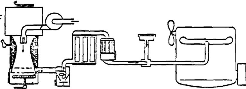
B. Wood gas apparatus for motor vehicle.
