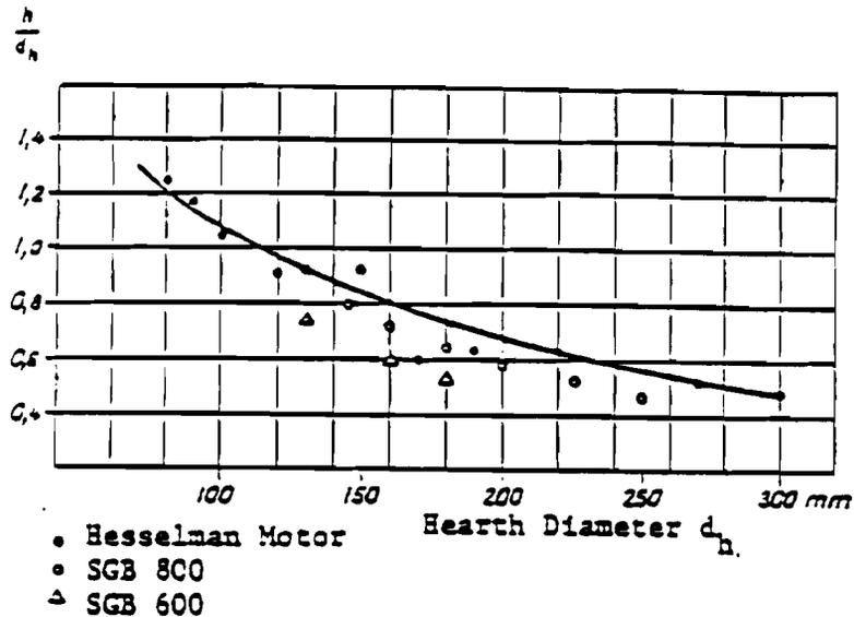
Figure 80. Height of the Nozzle Plane above the Hearth Construction for Various Generator Sizes.
