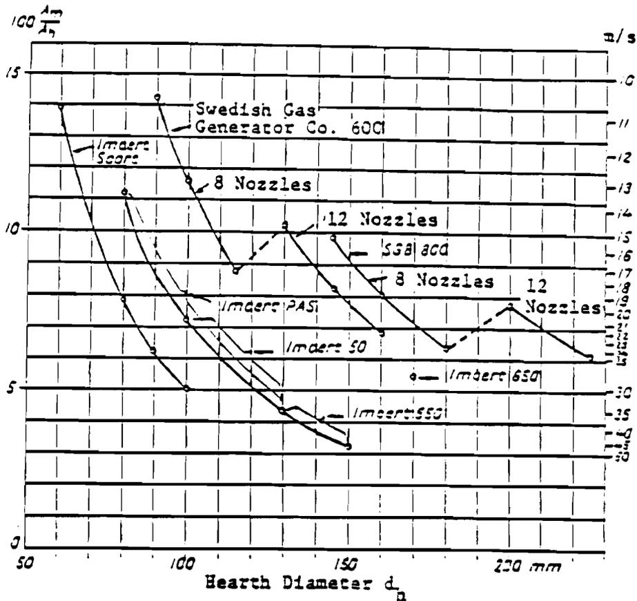
Figure 77. Graph Showing the Relation between the Total Nozzle Area and the Smallest Hearth Section, Air Velocity, etc., as a Function of Hearth Diameter at a Hearth Load of  $0.9 \text{ Nm}^3/\text{cm}^2\text{-hr}$ .
