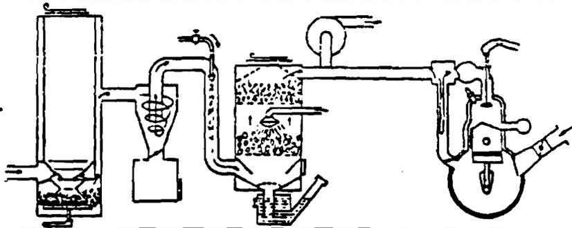
D. Wood gas apparatus with cloth cleaner and preheating of gas for motor vehicle.
