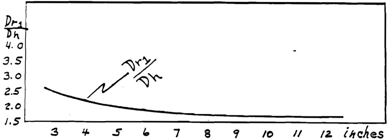
Figure 79 Diameter of nozzle ring opening (see appendix "C") diameter in relation to hearth constrictor ring diameter.
