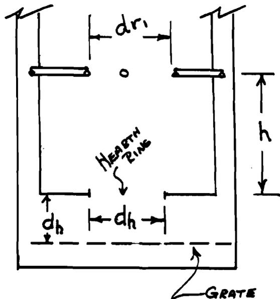
The nozzle opening circle diameter ( $dr_1$ ) is obtained from Figure 79. For this example, for a hearth diameter ( $d_h$ ) of 5.4, we pick off  $\frac{dr_1}{d_h} = 1.85$  or  $dr_1 = 5.4 \times 1.85 = 10$  in.
