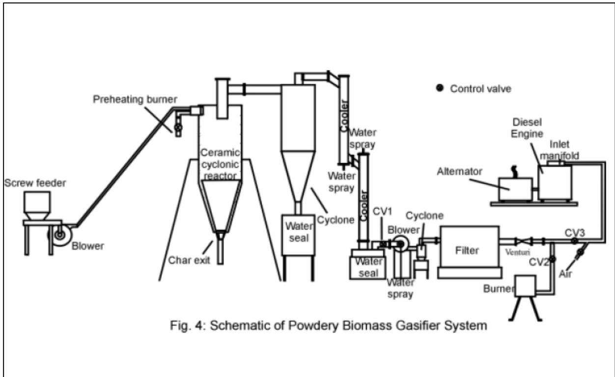
Fig. 4: Schematic of Powdery Biomass Gasifier System
