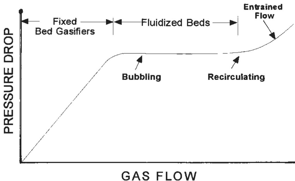
Fig. 5 Fixed and Fluidized Bed flow regimes for gasifiers
