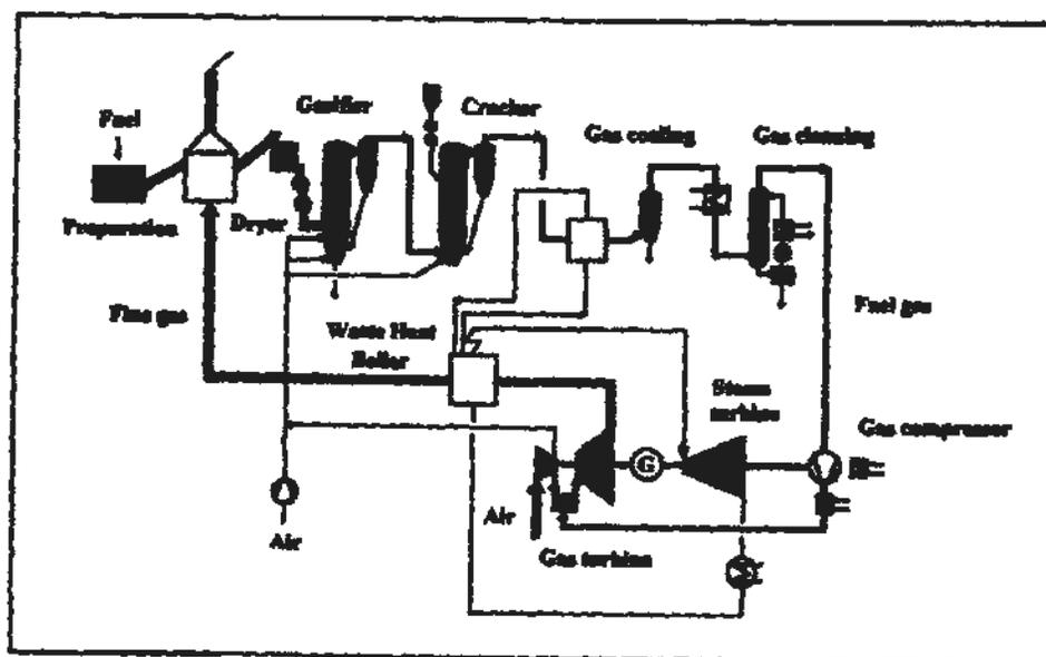
Figure 2 - TPS Biomass Integrated Gasifier Combined Cycle (BIG-CC) process system
