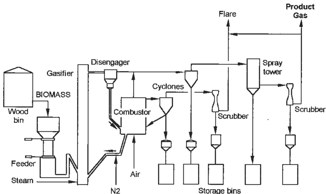
**Figure 1 - Battelle Columbus Gasification System**
