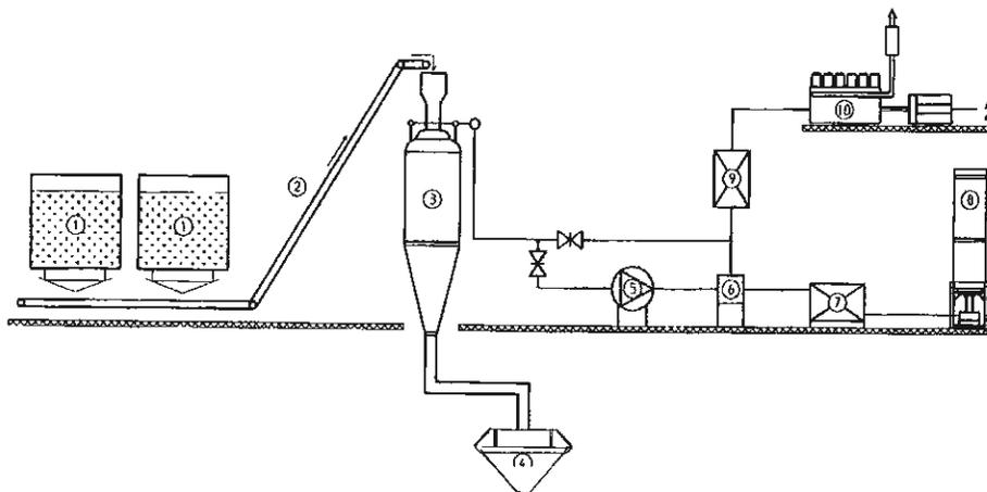
**Fig. 1. Schematic of HTV gasification plant showing (1) Fuel container, (2) Fuel feed, (3) Juch-Gasifier, (4) char-ash container, (5) flare fan, (6) condensate reservoir, (7) gas cooler, (8) Gas flare, (9) gas cleaning, (10) motor generator.**
