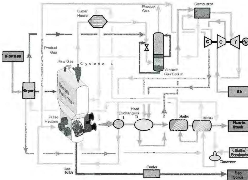
**Figure 3: Schematic of the Integrated Steam Reformer/Gas Turbine System for Biomass Power Generation**
