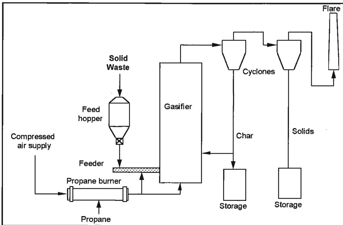
**Figure 1 - University of Sherbrooke/CQVB/Distech/Canmet 50kg/h Fluidized Bed Gasifier [Jollez, 1991]**
