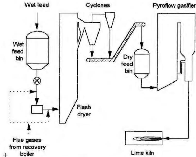
Figure 1 – Foster Wheeler Gasifier System
