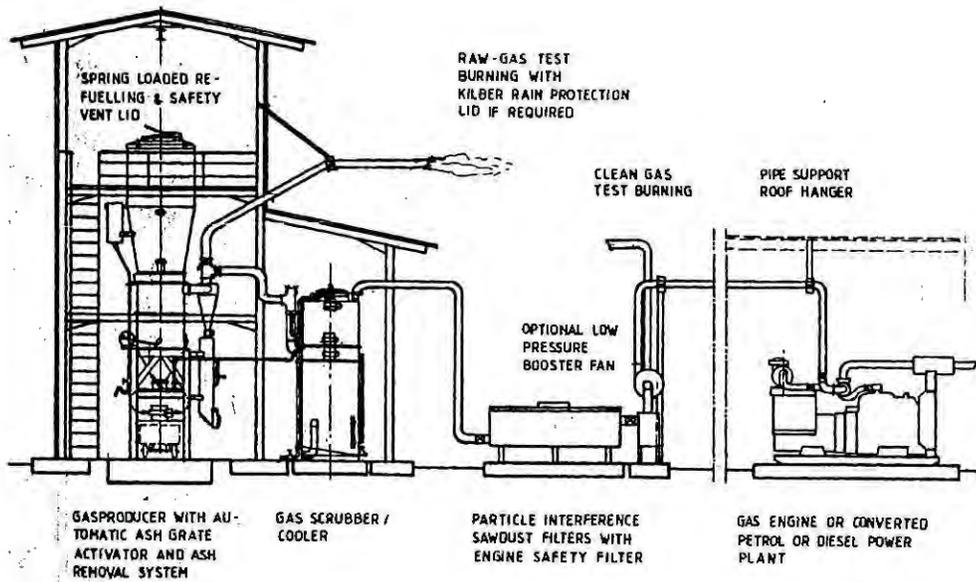
Fig. 2 – General arrangement of SJG gasifier for engine applications
