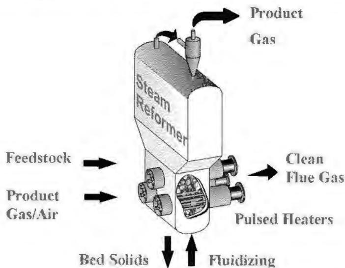
**Figure 1: PulseEnhanced™ Steam Reformer**
