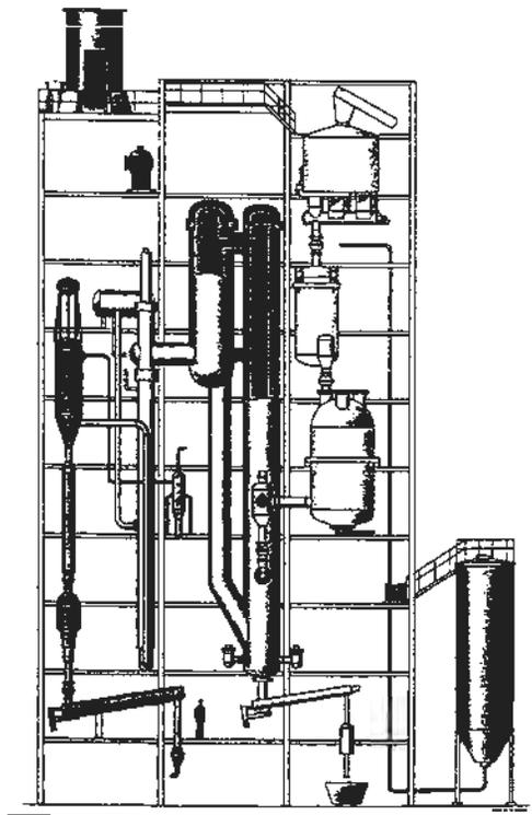
**Figure 2 - Arrangement of Varnamo IGCC plant (from report)**
