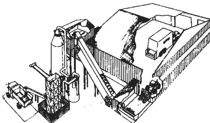
**Figure 1 Diagrammatic sketch of the Purox oxygen slagging gasification system**
