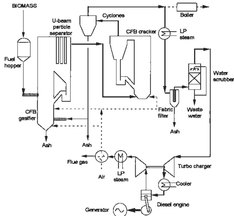
Figure 1 - Flowsheet of Studsvik Atmospheric Gasification Pilot Plant [Annon, 1992]
