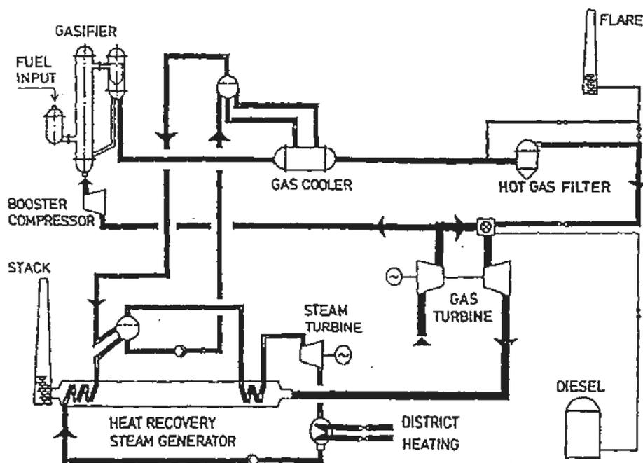
**Figure 1. - Layout of IGCC Varnamo plant**
