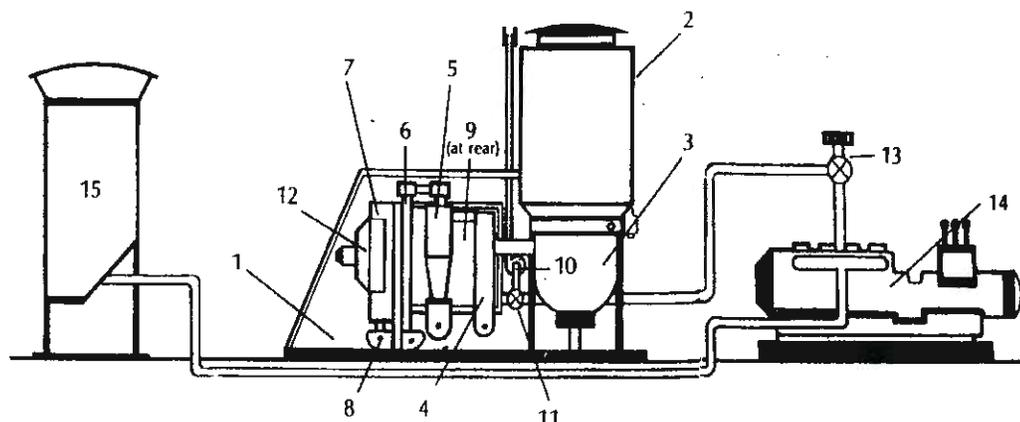
**Fig. 1 - Layout of typical Fluidyne gasifier plant showing (1) Supporting frame, (2) Wood fuel container, (3) Hearth, (4) expansion chamber (coarse particles), (5) Multi Cyclone, (6) saturating cooler, (7) condensing cooler, (8) condensate tank, (9) volume filter, (10) start-up fan, (11) change-over valve, (12) gas cooler fan, 13 engine gas/air mixer controller, (14) engine/generator set, (15) wood drier using waste heat.**
