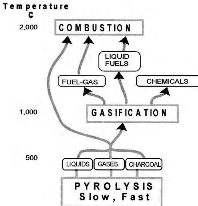
**Fig. 1 - Pyrolysis (at 500 °C) yields liquid, gaseous and charcoal products which can be gasified (1,000°C) to yield a fuel gas, liquid fuels or chemicals; or the products (gases, vapors and charcoal can be burned directly for heat (2,000 °C) .**
