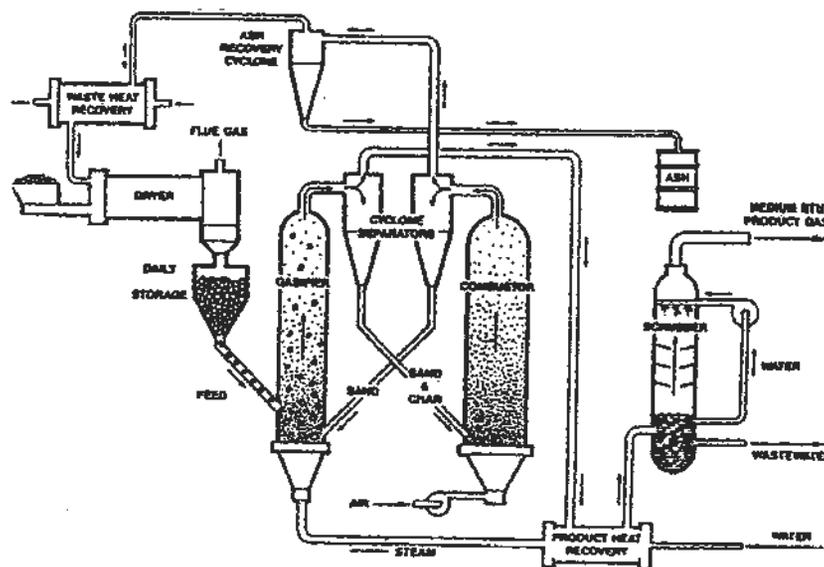
Figure 1 - Diagram of Burlington fluidized bed gasifier system for production of medium energy gas without an oxygen plant
