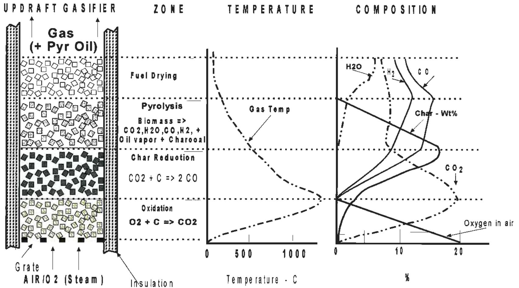
Fig. 2- Schematic diagram of an updraft gasifier showing the gasifier zones, the reactions, the temperatures and the gas composition (zone height not necessarily to scale). Air or oxygen passes up through a grate and burns charcoal, generating very high temperature CO<sub>2</sub> in the oxidation zone; the CO<sub>2</sub> is then reduced to CO (endothermic, gas cools) in the reduction zone; the hot gas then pyrolyses and dries the incoming fuels.
