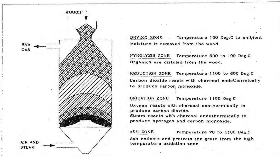
Fig. 2 – Schematic of reaction zones in Wellman Gasifier
