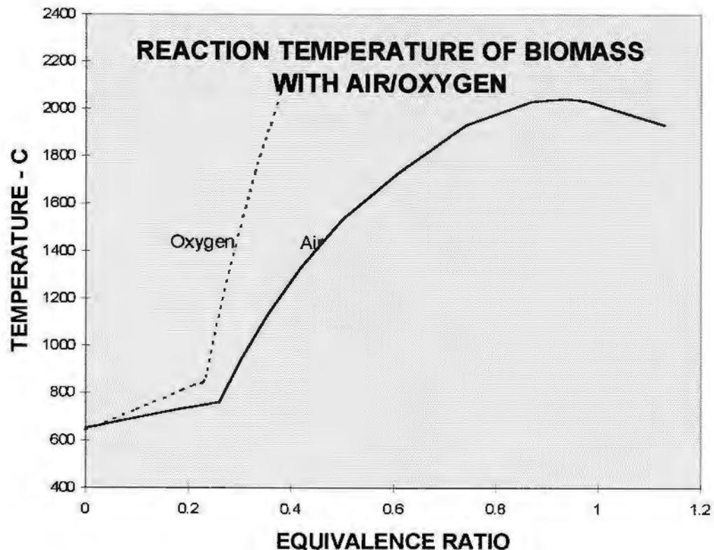
Fig. 7 - Temperature of the reaction of dry biomass with air or oxygen as a function of equivalence ratio
