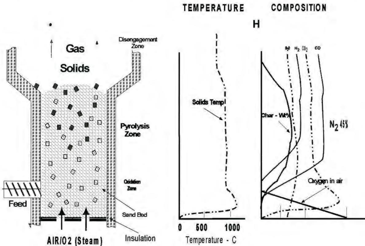
Figure 6 - Schematic diagram of a fluidized bed gasifier
