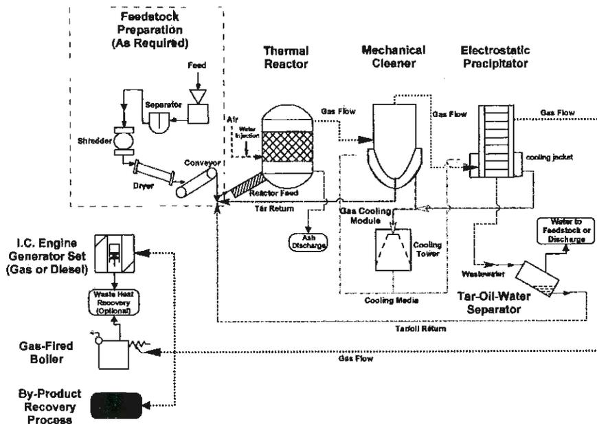
Fig. 2 – Thermogenics #103 Process Flow Sheet for electrical power, steam generation or by-product recovery
