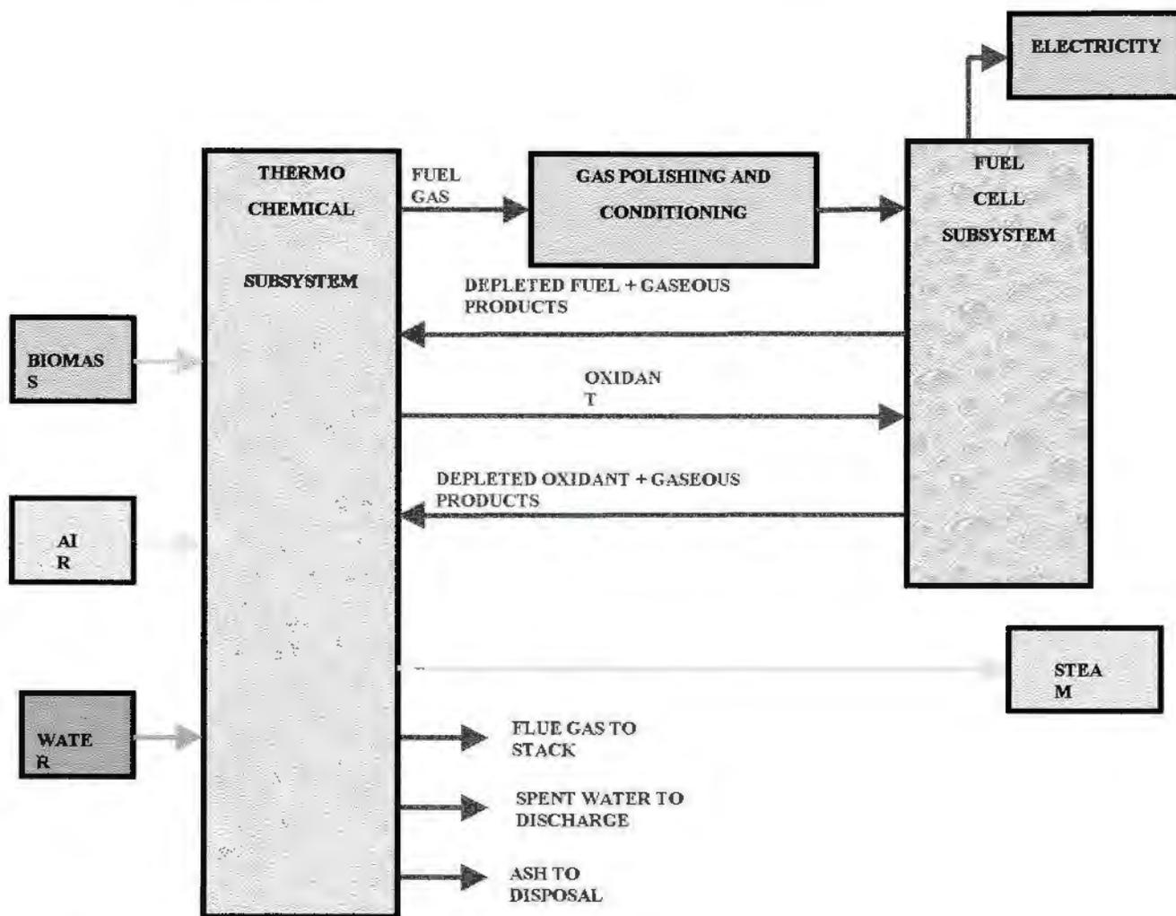
**Figure 4: A Simplified Block-Flow Diagram Of The Thermochemical System**
