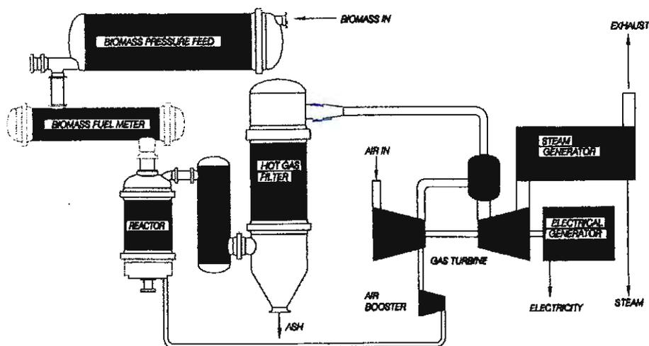
Figure 1 – Block Diagram of Cratech Process
