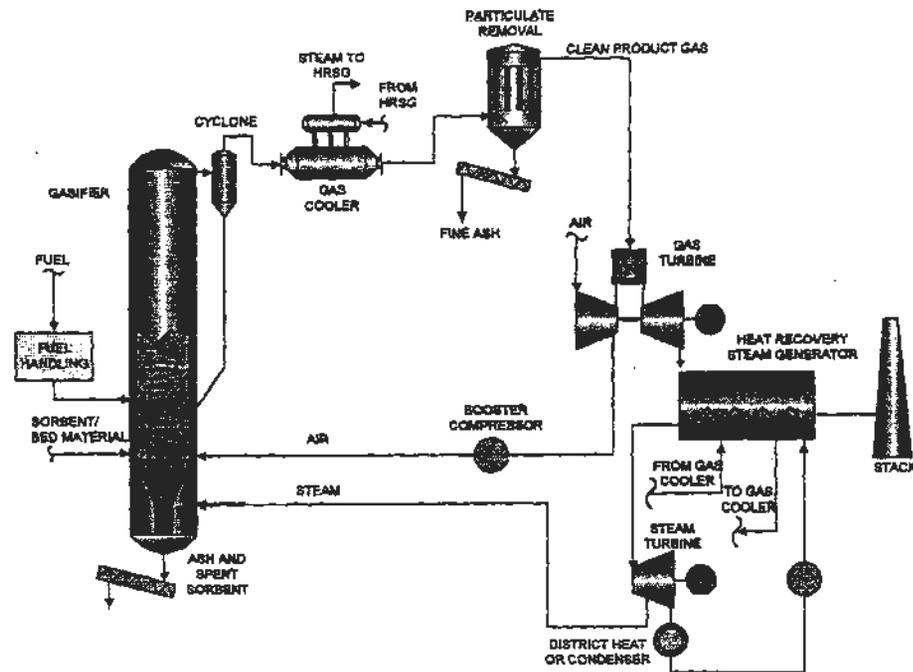
Fig. 1 Carbona Pressurized Fluidized Bed Gasifier (I will use your figures here)
