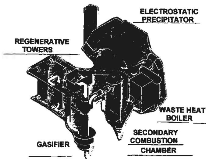
Figure 1 - Flowsheet of Sofresid/Caliqua (Andco Torrax process) MSW Gasification System at Créteil [Bridgwater, 1993]
