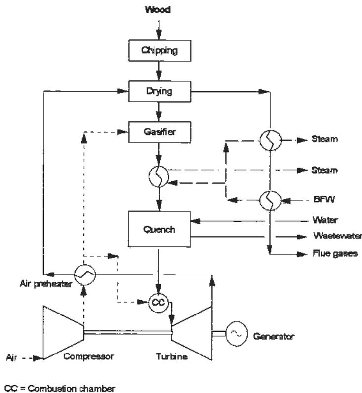
Figure 2 - Lurgi Gas Turbine Heat and Power Cogeneration Scheme [7]
