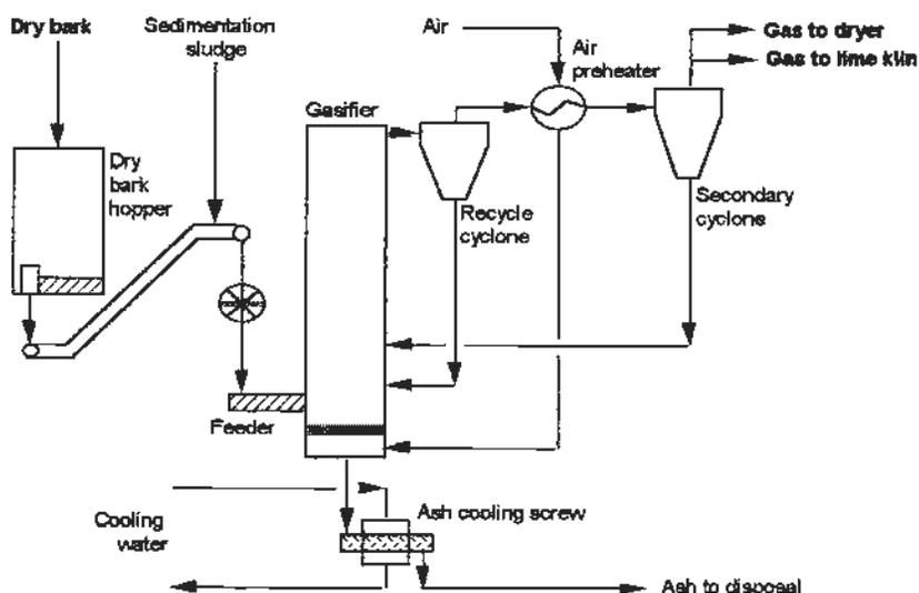
Figure 1 - Lurgi CFB Gasification System at Pöls Pulp Mill [Herbert, 1989]
