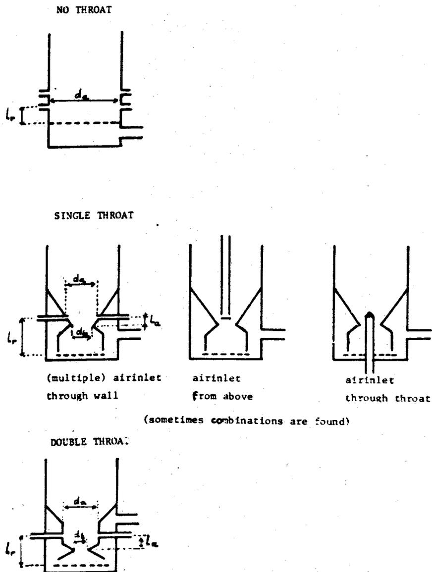
*Figure 2: The different designs for co-current gasifiers, with the characteristic measures;  $d_t$ : throat diameter,  $d_a$ : diameter at air inlet,  $L_r$ : reduction zone length,  $L_a$ : height of air inlet above throat.*
