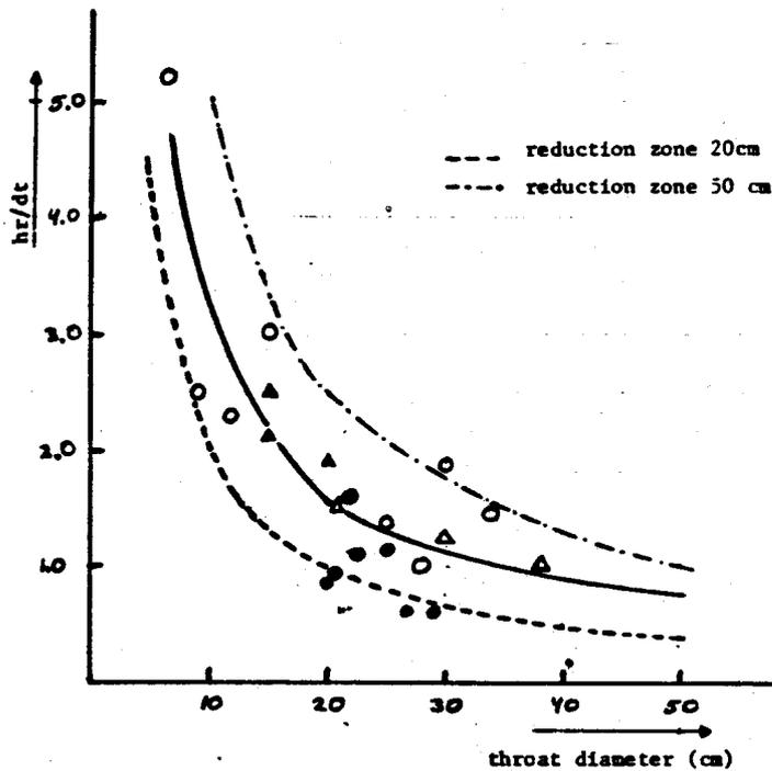
Figure 5:  $h_r/d_t$  versus throat diameter ( $d_t$ ).
