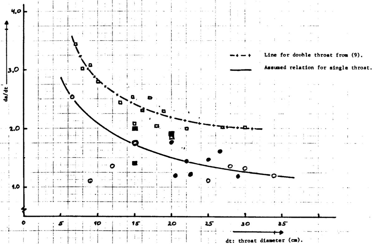
Figure 7: Ratio of diameter of air inlet and throat ( $d_a/d_t$ ) against capacity (given as throat diameter).
